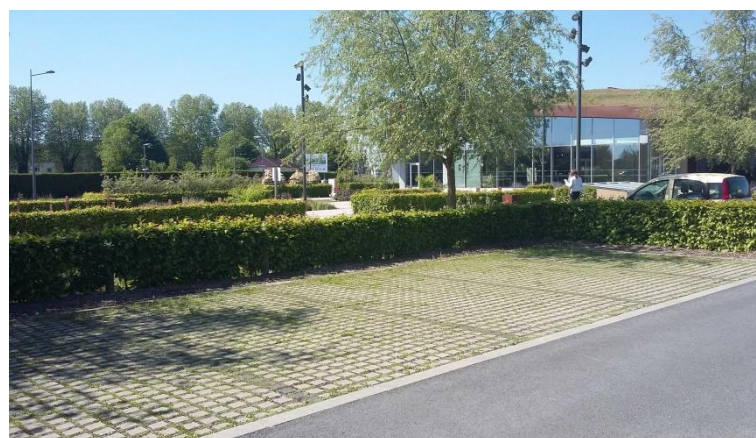
Figure 22: Illustrations de techniques alternatives – matériaux drainants
